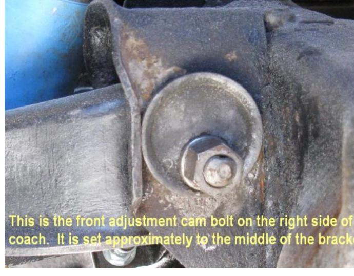
Torque the cam nut to 80 ft-lbs. Hold a wrench on the cam bolt head to keep the cams from turning.
