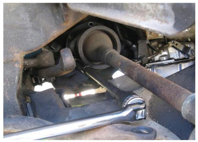
Remove the caliper bolts with a <u>3/8" hex wrench</u>. Remove any other brackets or <u>cable ties</u> holding the flexible brake line. Slide the caliper off the rotor. If it's stuck, you may need to use a big C-clamp to retract the piston (see manual). and let them hang there.
