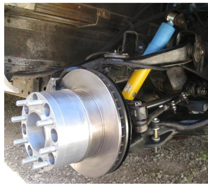
The classic 1973 - 1978 <u>GMC</u> Motorhome is a marvelous machine. However, as most GMC owners know, the front end is a weak point of the design. Around 2007, Bill Hubler developed a kit to retrofit GM heavy duty truck parts onto the GMC motorhome front end. In 2011, Manny Trovao figured out how to improve the kit and brought the cost down by buying new parts in large quantities. The result is the new Version II One-Ton Front End Kit.
