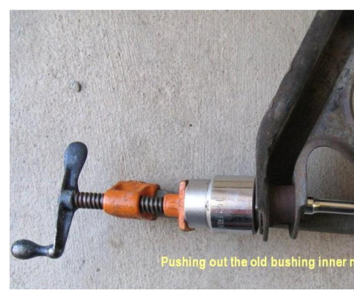
Once the sleeve is out, turn the socket and extension around and use the 3/4" socket to push out the rubber bushing. Do not damage the outer sleeve on the front of the arm since you'll need to reuse it with the new bushing.
