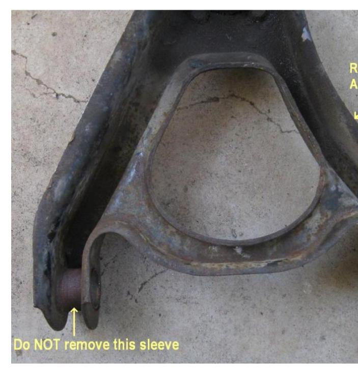
Use a hammer and punch to deform the cut sleeve and drive it out of the A-arm.
