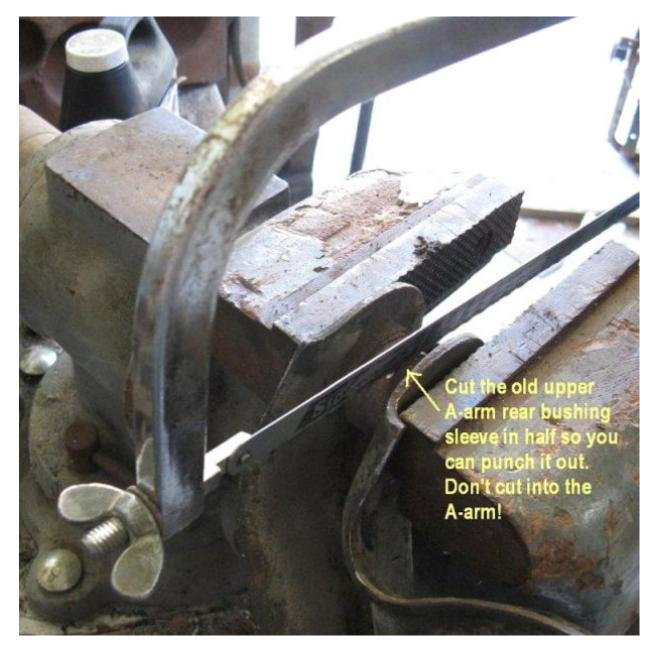
If you get them mixed up, the rear of the upper A-arm is the one with the curved side. Do not remove the front sleeve since you'll need to reuse it for the new urethane bushing.
