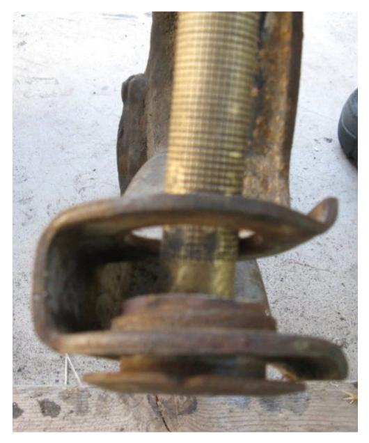
Clean up the rear hole in the arm really well and remove any burrs, rust, paint, or dirt. It may help to lightly sand or file the hole, but don't remove too much metal. Align the new offset bushing in the rear hole of the upper A-arm with the arrow pointing AWAY from the ball joint.
